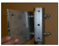
C) Install tube reinforcement in head assembly
