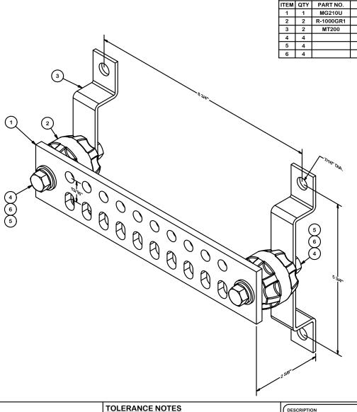
TOLERANCES ON DIMENSIONS, UNLESS OTHERWISE NOTED ARE: SAWED, SHEARED AND GAS CUT EDGES (\$ 0.030") - NO CONING OF HOLES LASER CUT EDGES AND HOLES (\$ 0.030") - NO CONING OF HOLES
