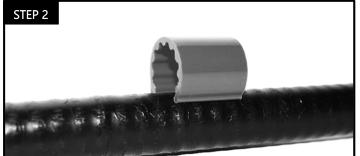
Align the TEK  $Clip^{TM}$  with the opening against the cable where it is to be installed. Ideally, 5 inches or more from the end of the cable to allow for weatherproofing.
